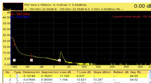
Figure 10. OTDR Test with 6 cm Sleeve Protection one connection
