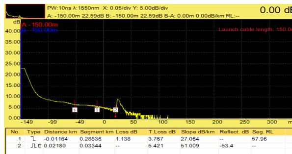
Figure 8. Testing of OTDR with Sleeve Protection 4 cm one connection
