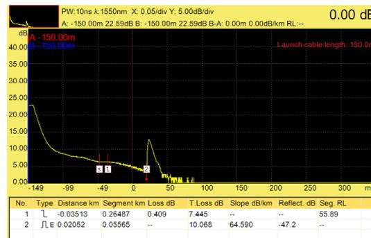
Figure 11. Testing OTDR with Sleeve Protection 6 cm two
