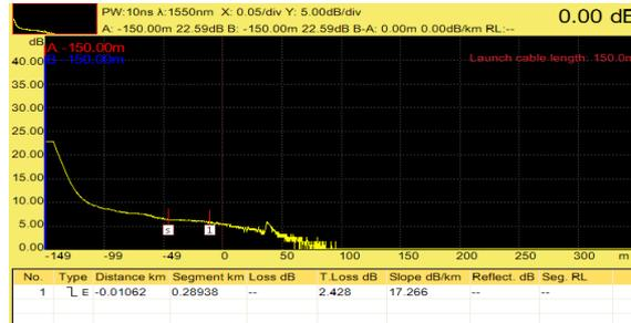
Figure 7. OTDR Test Without Connection
