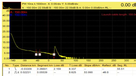
Figure 9. Testing OTDR with Sleeve Protection 4 cm two joints
