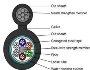
Figure 3. Basic Construction of Aerial Cable
