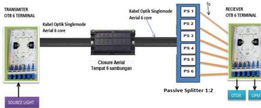
**Figure 6.** Design of transmission attenuation measurement of Single Mode Aerial Fiber Optic Cable using a passive splitter
